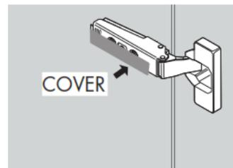
After adjustment, fit the Ab covers onto the other hinges
