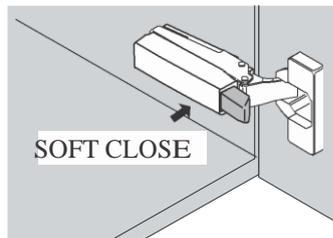
After adjustment, fit 1 soft close per door and not 1 per hinge
