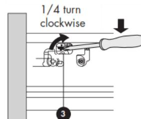
Insert the screwdriver in the cross slot and lift up the flap
